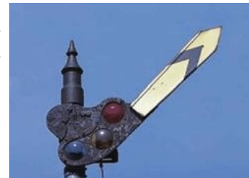
Upper quadrant semaphore signal. This signal is displaying the same indication as the lower quadrant signal above.
