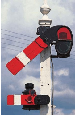
Lower quadrant semaphore signal. Upper head indicates this signal may be passed, and lower head indicated the next signal may not be passed.
