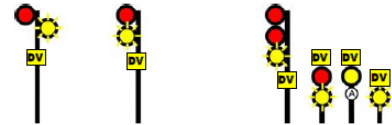
429. Diverging to Stop - Proceed, DIVERGING speed passing signal and through turnouts, preparing to stop at next signal.
