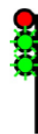
417. Limited to Limited - Proceed LIMITED speed passing signal and through turnouts, approaching next signal at LIMITED speed.
