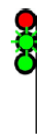
418. Limited to Medium - Proceed LIMITED speed passing signal and through turnouts, approaching next signal at MEDIUM speed.
