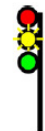
433. Slow to Medium - Proceed SLOW speed passing signal and through turnouts, approaching next signal at MEDIUM speed.
