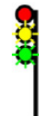
432. Slow to Limited - Proceed SLOW speed passing signal and through turnouts, approaching next signal at LIMITED speed.
