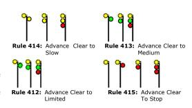
Each indication is displayed when the SGA's inputs have the  ${\bf AV}$  input active along with the necessary DCA and speed restriction inputs corresponding to the non-Advance version of the indication. See the indication Truth Table for the mode you are using (CTC or ABS), available on our website under Product Documentation.
