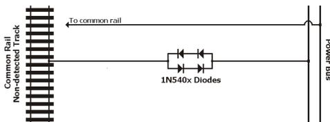
To avoid this change in speed, non-detected track should have its power pass through a pair of diodes that are in parallel with another pair with the opposite polarity. Diodes used should have suitable current carrying capabilities for the application.
