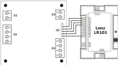
The LR101 from Lenz has eight active-low inputs, labeled from 1 to 8. Each output of the Quad Occupancy Detector may connect to any one of the eight inputs on the LR101.
