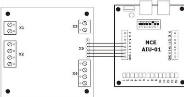
The AIU-01 Auxiliary Input Unit from NCE works well with the Quad Occupancy detector, though there is a known issue with inputs 6 and 7 at this time, described below.
