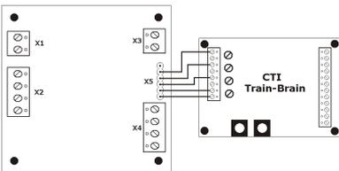
Each of the four inputs on the Train-Brain have two terminals, labeled 'A' and 'B'.
