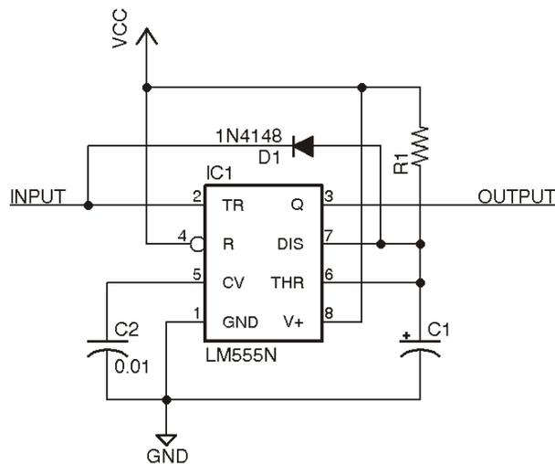
The only issue with this circuit is that it inverts the occupancy logic states. The output will be high when the track is occupied and low when unoccupied. This can be worked into the design of the circuit it drives or configured if it feeds a software system, or an inverting gate can be added to the output to restore an active low output.
