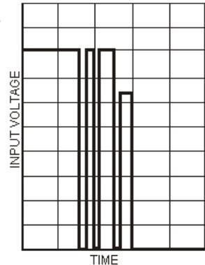
With an occupancy detector, bounce is magnified by track conditions. Slightly dirty sections of track can add to bounce noise. Momentary loss of detection can even be substantial enough to have an effect when driving a relay circuit. The Quad Occupancy Detector from Circuits4Tracks counters the effects of momentary loss of detection with the use of a capacitor on its output, but bouncing will still occur when the state changes from unoccupied to occupied and back again.
